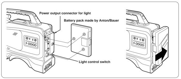
■ Provided on the battery holder made by Anton/Bauer are a power output connector for a light and a light control switch. A light can be easily attached. For details on lighting systems, consult an Anton/Bauer representative.
